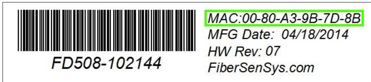
Figure 2: Hardware (MAC) address on the APU's barcode ID label.
