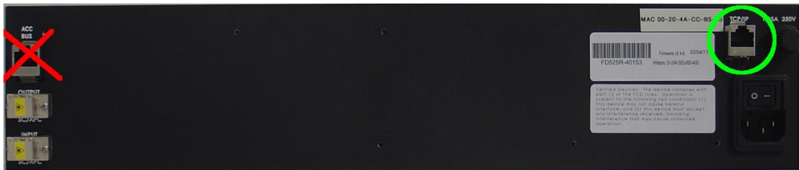
Figure 14: Ethernet Port on the back of the FD525R
