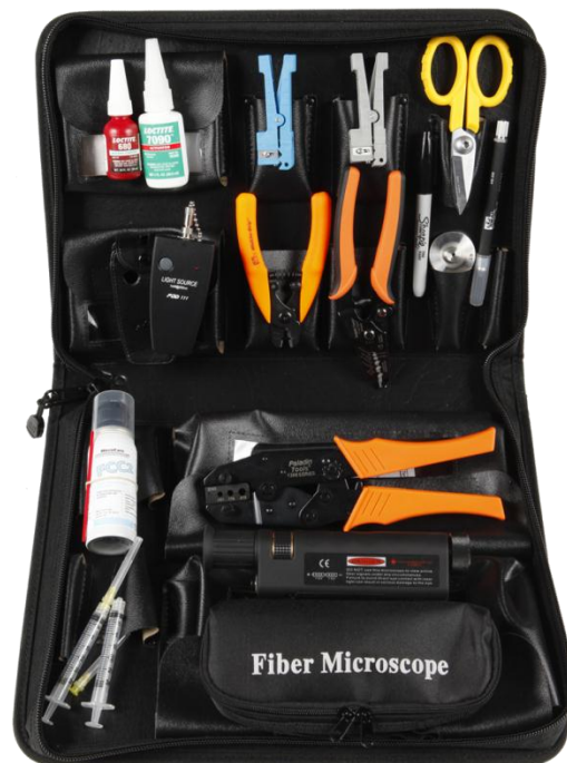
Figure 4-1. Basic termination kit, for installing connector termination.
