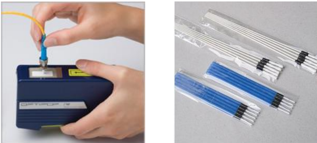
Figure 6-1. An example of a mechanical cleaner (left), used for cleaning the ends of the ferrules on connectors. Also, an example of swabs (right) used to clean the insides of feed-through couplers.
