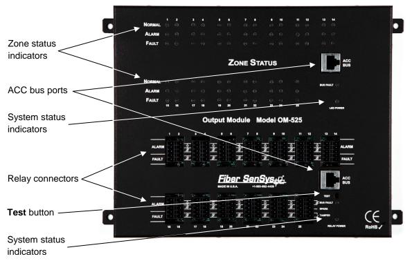
Figure 1. OM525 output module, top view
