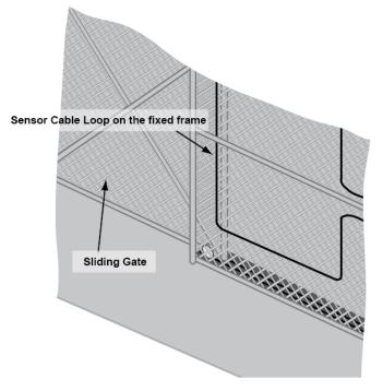
Figure 6: Sensor cable deployment on a sliding gate
