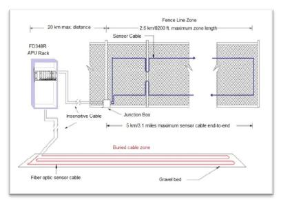
Figure 2: rack-mounted FD348R APU and fence / buried installation
