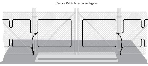
(Sensor Cable in solid conduit under the roadway)
