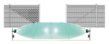
access points. Bi-state microwave barrier curtains offer an effective intrusion detection solution at gate entry points. Volumetric microwave detection systems can provide an alternative to swing gates
