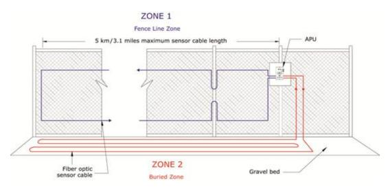
Figure 1: Field mounted FD300 series APU head-end with dual -zone configuration, fence mounted sensor cable & buried zone
