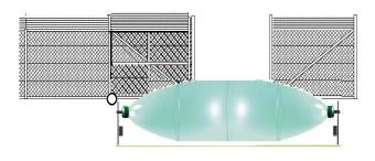
or sliding gates, and sensors protect gate areas with a system that contains fewer moving parts and can operate reliably longer and with less maintenance. Volumetric sensors are easy to install, especially for existing facilities where protection is desired without a re-design of the fence system. Precautions are necessary in microwave
