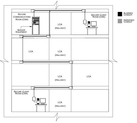
Figure 8 - Alarmed segments of a "hardened" carrier
