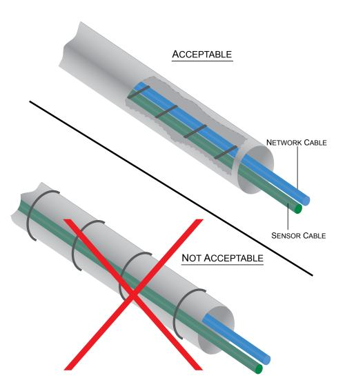
Figure 14 - Alarming a carrier with the sensor cable
