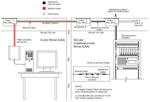
Figure 9 - SecurLAN<sup>®</sup> cable deployment scheme
