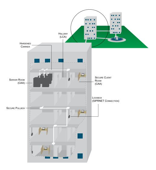
Figure 1 - Basic PDS Components
