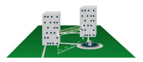
Figure 3 - Building - to - building PDS construction options
