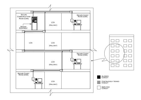
Figure 7 - Example alarmed carrier layout
