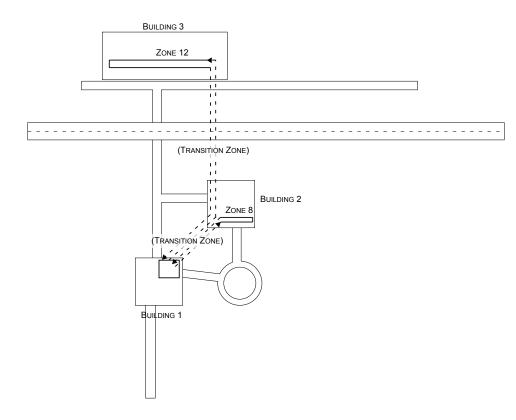
Figure 13 - Transition zones in a multi-building layout
