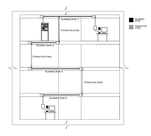
Figure 11 - Transition zones in an alarmed PDS
