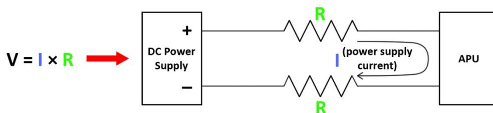
The voltage drop ( $V$ ) across each leg of the wiring is equal to the power supply current ( $I$ ) flowing in the wire multiplied by the wire’s resistance ( $R$ ).
