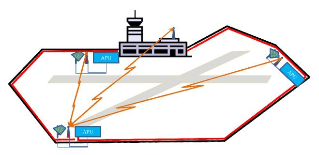
Figure 1. The APU (housing electronics and optics) senses disturbances at the perimeter, along the optical fiber. Alarms created by these disturbances are communicated wirelessly to the head end in the airport terminal. Remote electrical power (either solar or thermo-electric) powers the wireless modem and the APU.
