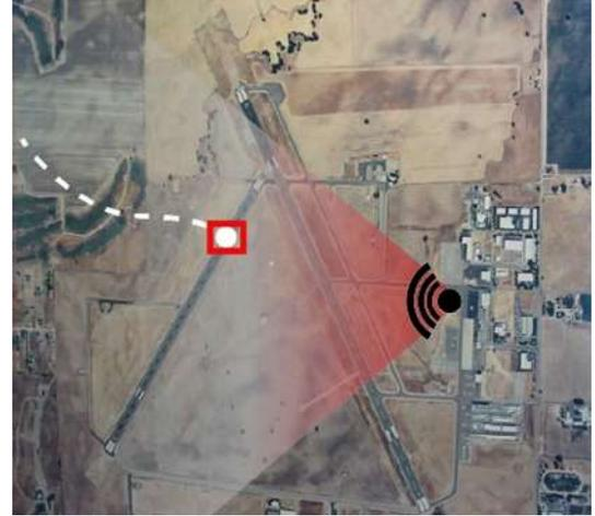
Fiber SenSys, Inc. has partnered with **SpotterRF** to reach beyond the fence line or where no fence exists to provide the market's best solution for early notification of intruders in a large area. SpotterRF systems identify multiple simultaneous targets and provide a trail indicating the intruders' paths.
