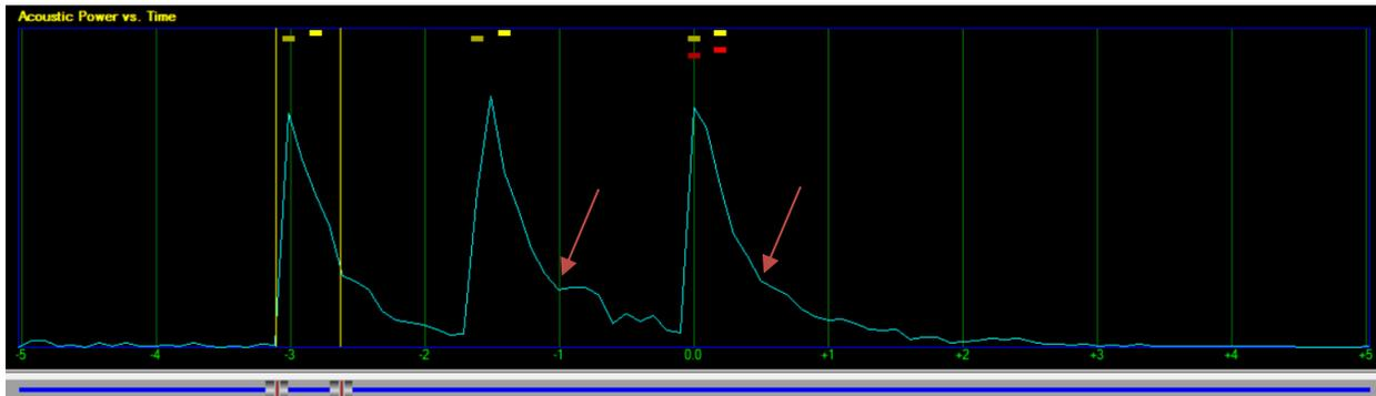
Figure 12 – Arrows indicate signal decline for measuring Duration
