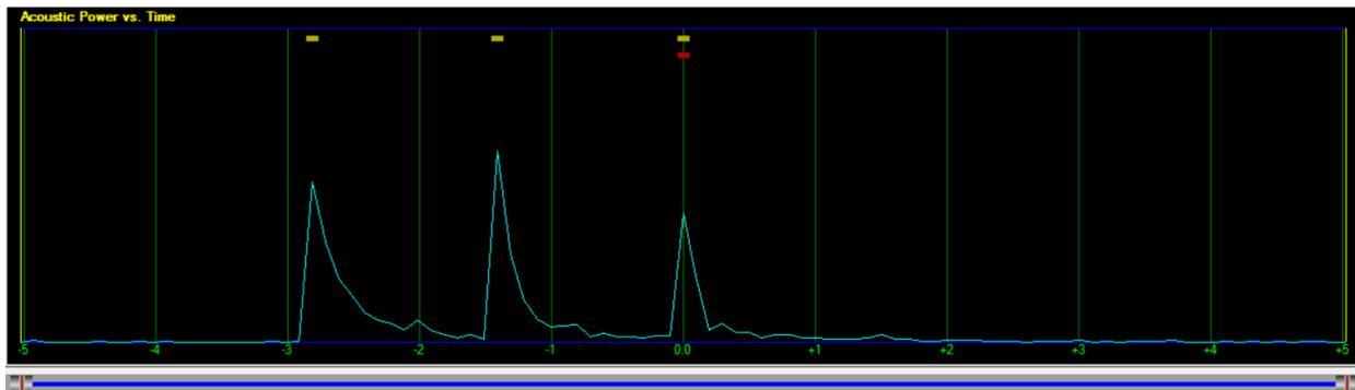
Figure 13 – Cut simulation generates alarm only on P2
