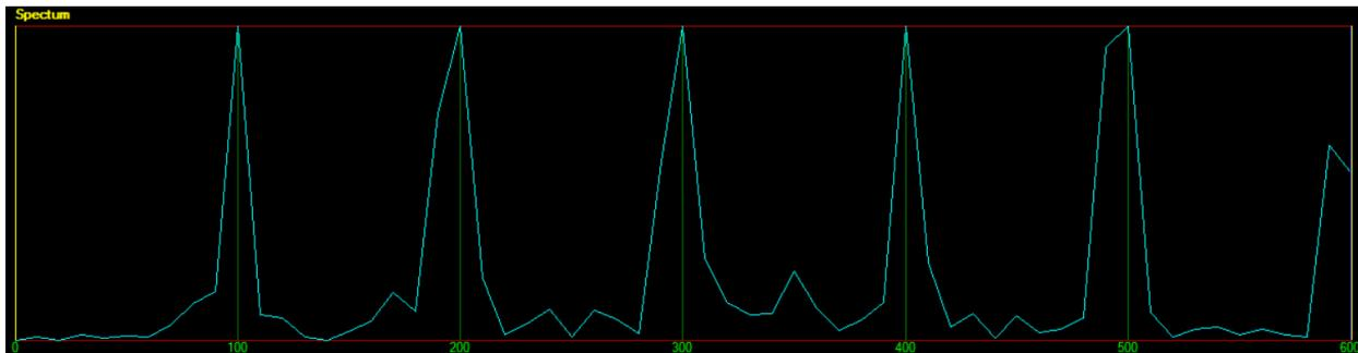
Figure 7 – Nuisance source generating harmonic frequencies of 100Hz
