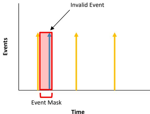
Figure 4 – Event mask time prevents excessive events from being generated
