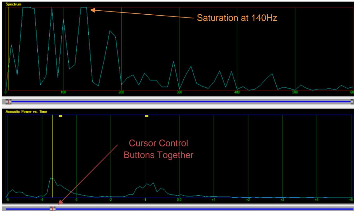
Figure 9 – Intrusion signal with saturation up to 140Hz
