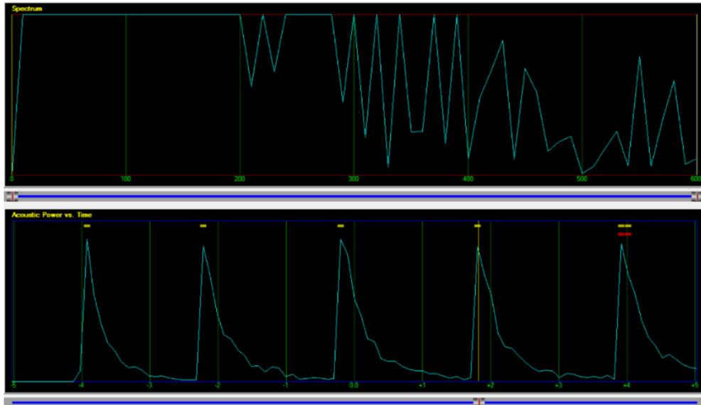
Figure 11 – Intrusion signal saturation at ~400Hz
