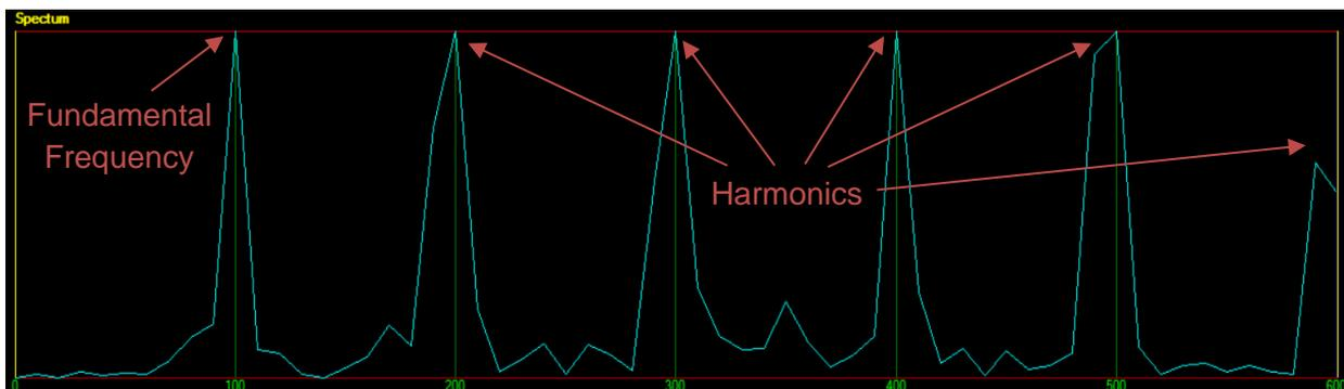
Figure 15 – 100Hz harmonic frequency response
