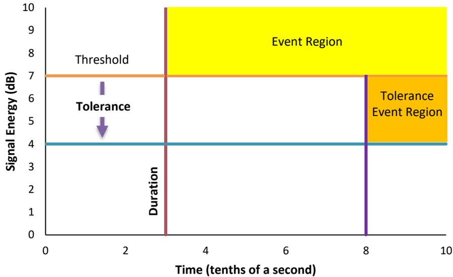
Figure 3 – Threshold, Duration, and Low Level Tolerance diagram
