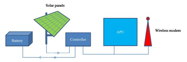
Figure 2. The solar-powered module consists of solar panels that charge batteries used to run the APU and wireless modem. A controller optimizes the charging process. The batteries are designed and sized to store enough energy to power the system during nighttime and seasonally expected periods of cloud cover.
