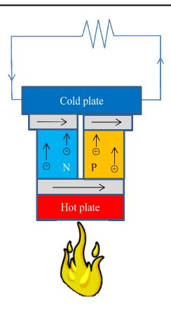
Figure 3. The TE generator uses heat, applied to a specially designed semiconductor junction, to generate electrical current. Because the AD-525 is so efficient a single 500-gallon buried propane tank holds enough fuel to run the system for an entire year.
