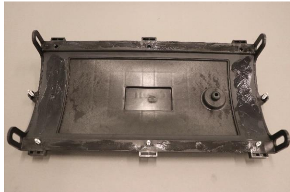
Figure 59. Silicone grease around outer edges of the cover gasket
