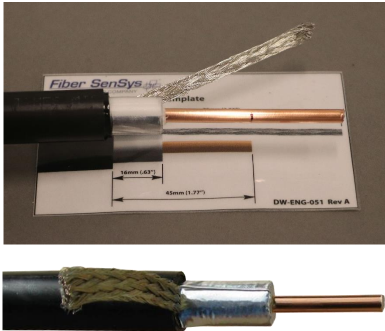
Figure 48. Marking the center conductor (top); the finished center conductor cut to length (bottom)
