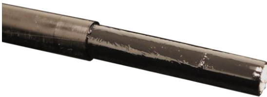
Figure 43. Sensor cable with outer jacket removed and cleaning process
