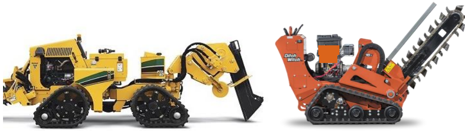
Figure 15. Cable Plow (left) and Walk-behind Trencher (right)
