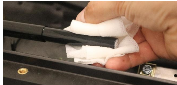
Figure 43. Sensor cable with outer jacket removed and cleaning process
