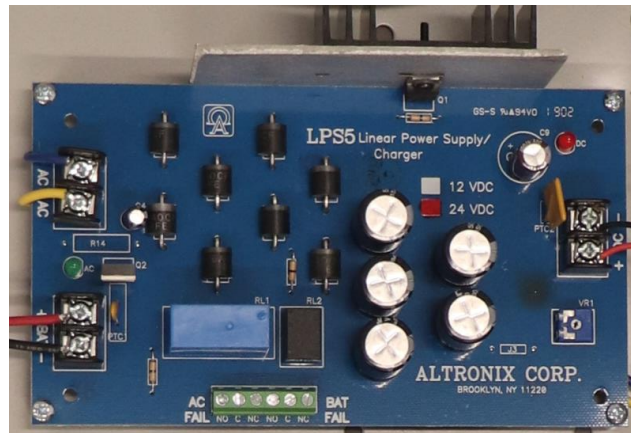
Figure 68. Linear Power Supply (LPS5)
