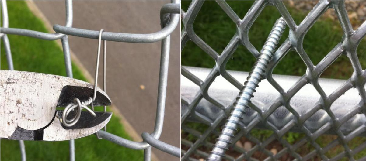
Observe using a stainless steel wire tie for a cut test and using a threaded bolt for a hacksaw test
