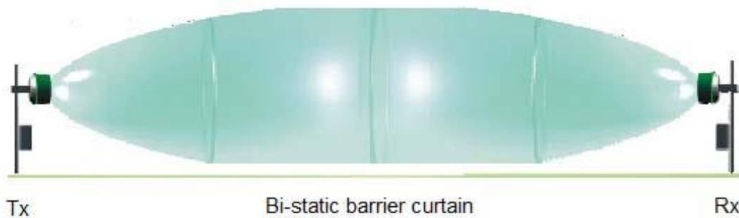
Figure 4: Volumetric microwave barrier curtain models range from 50 m to 500 meters.
