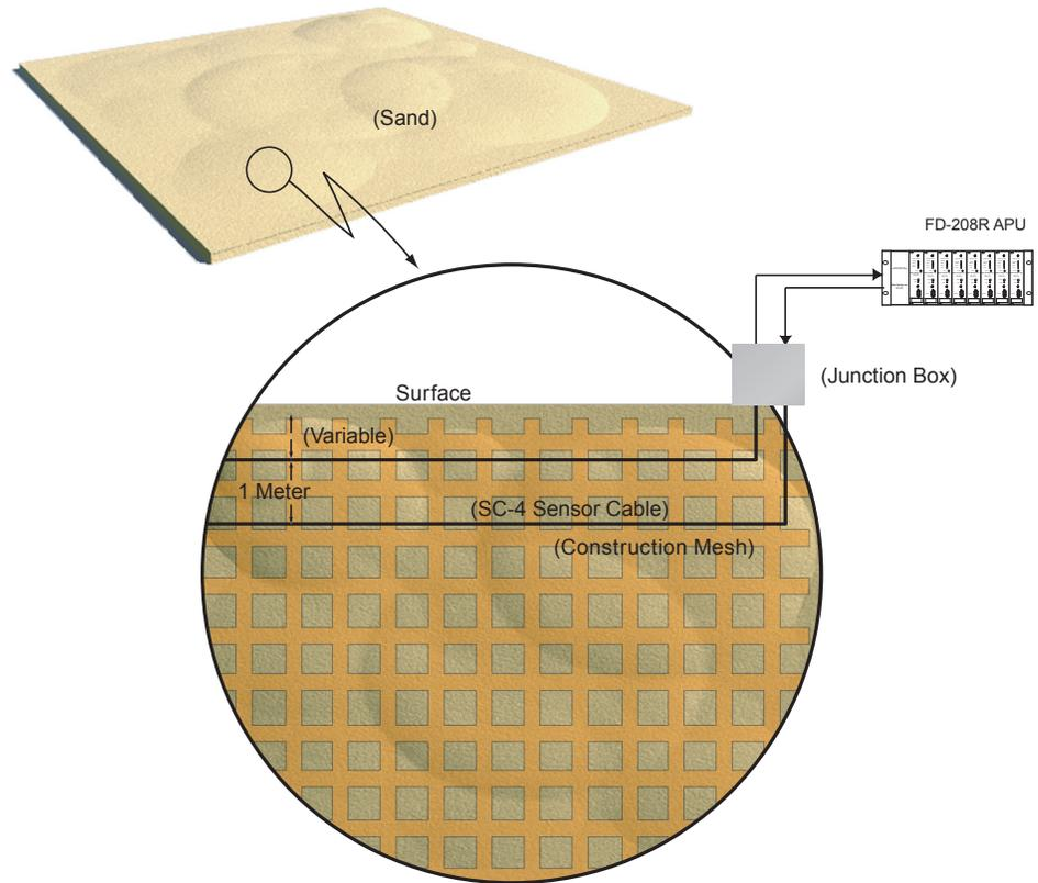
Figure 3 - Protecting against tunneling-type intrusions
