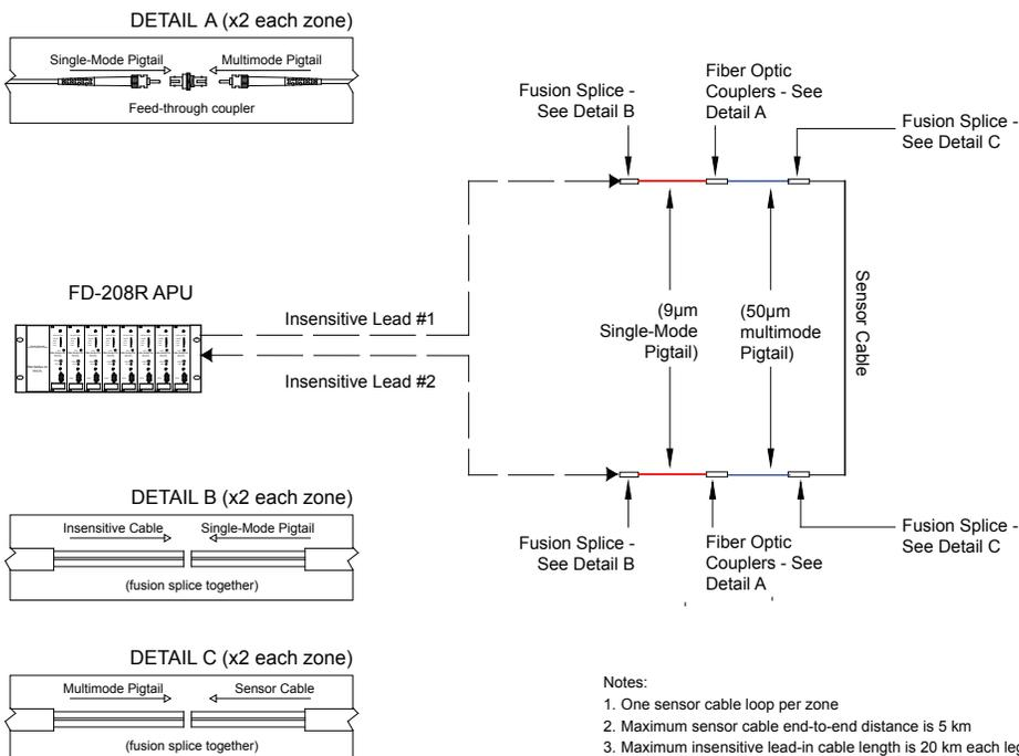
Figure 1 - Connecting sensor cable to insensitive leads using pigtails
