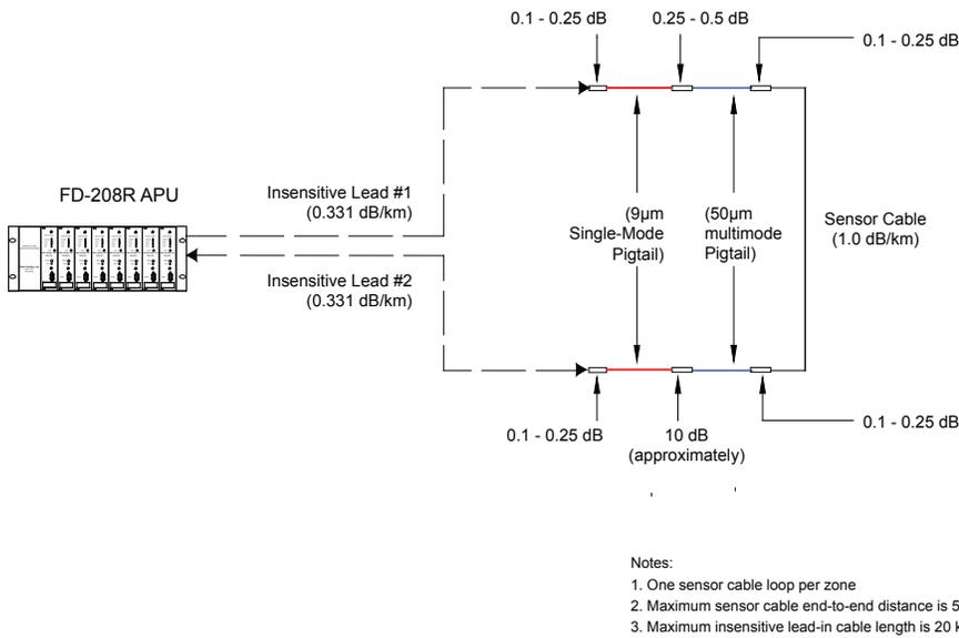
Figure 2 - Optical losses associated with the FD-208 and FD-340 series
