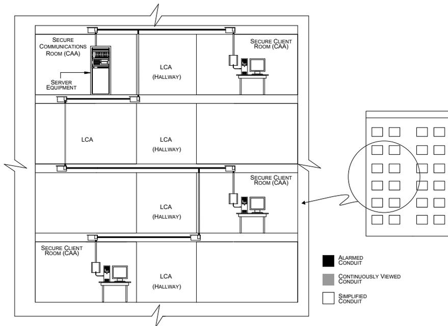
Figure 7 - Example alarmed carrier layout
