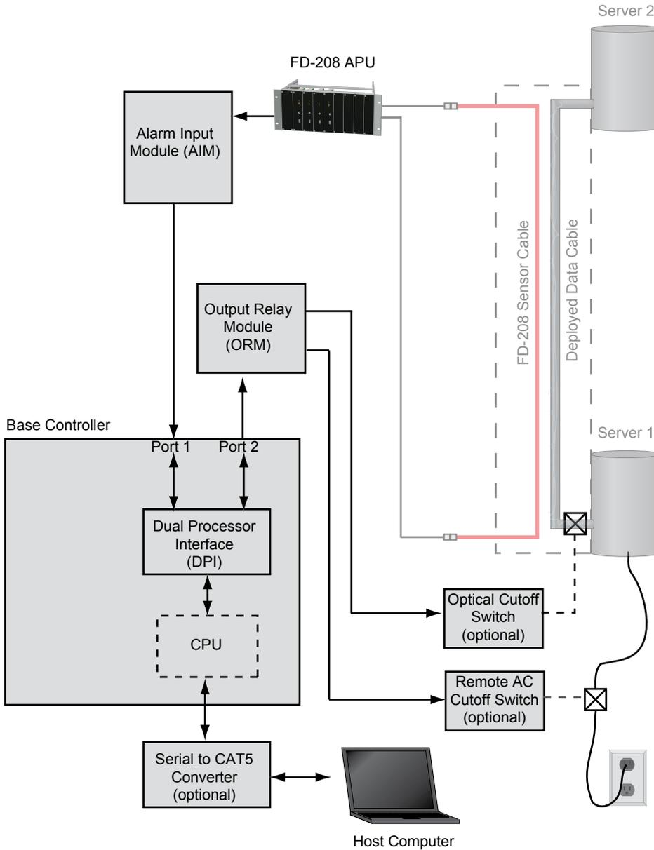
Figure 6 - SecurLAN® component block diagram
