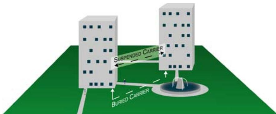
Figure 3 - Building - to - building PDS construction options
