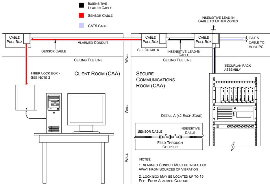
Figure 9 - SecurLAN<sup>®</sup> cable deployment scheme
