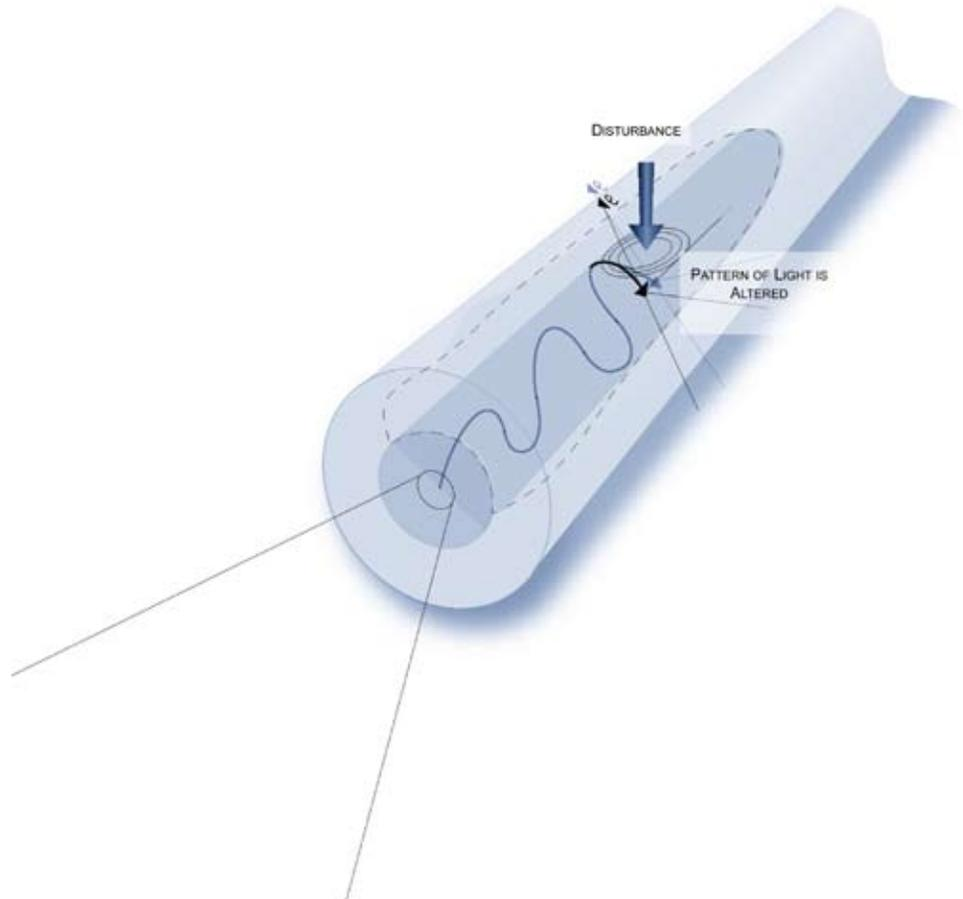
Figure 5 - Effects of vibration on the sensor cable
