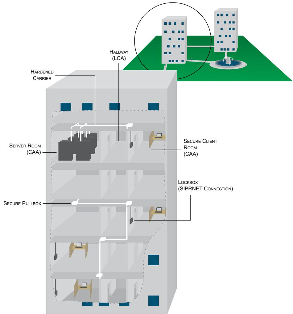
Figure 1 - Basic PDS Components
