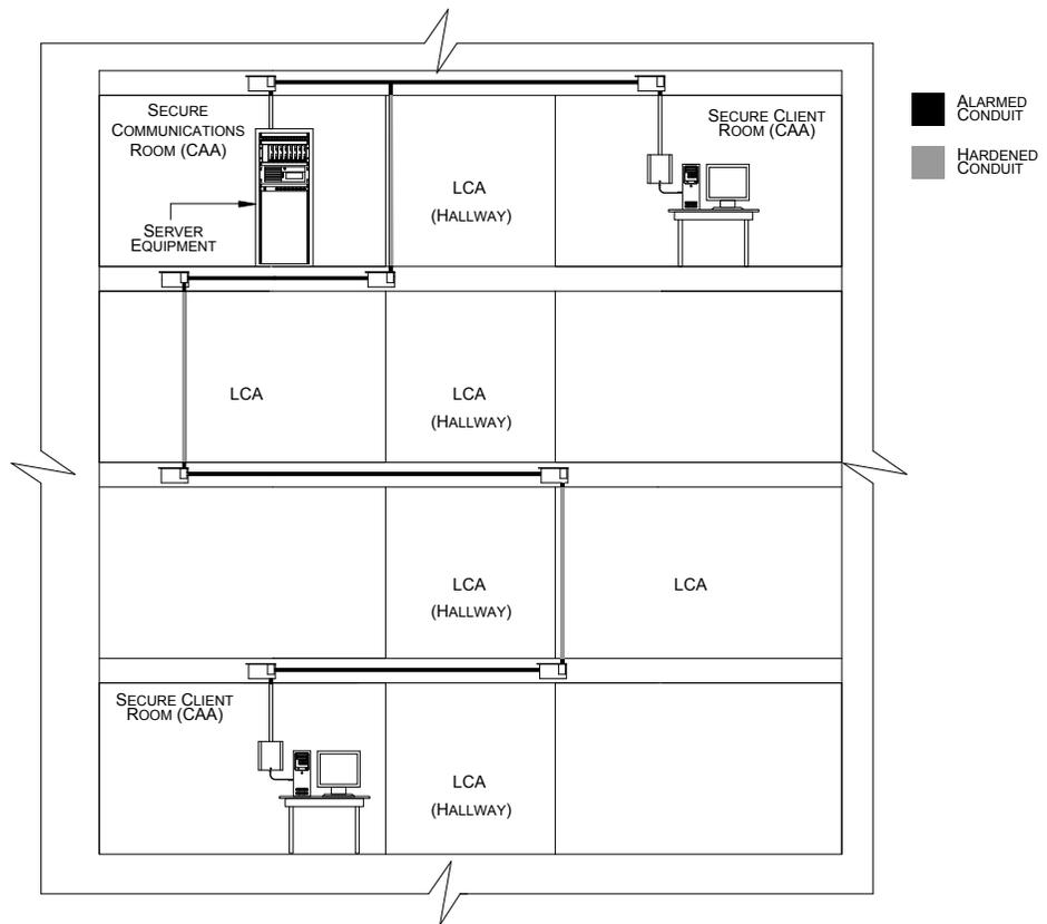
Figure 8 - Alarmed segments of a "hardened" carrier
