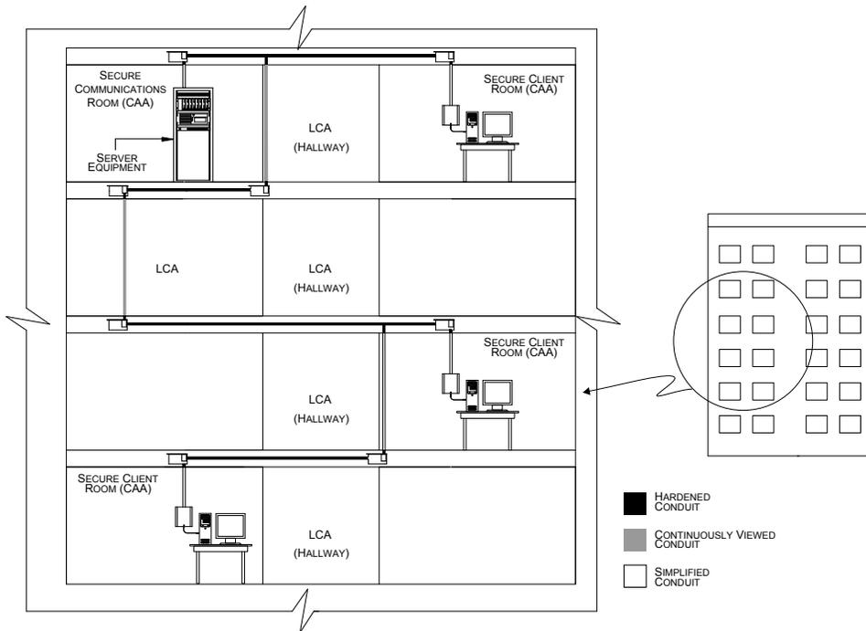
Figure 2- Single building PDS layout
