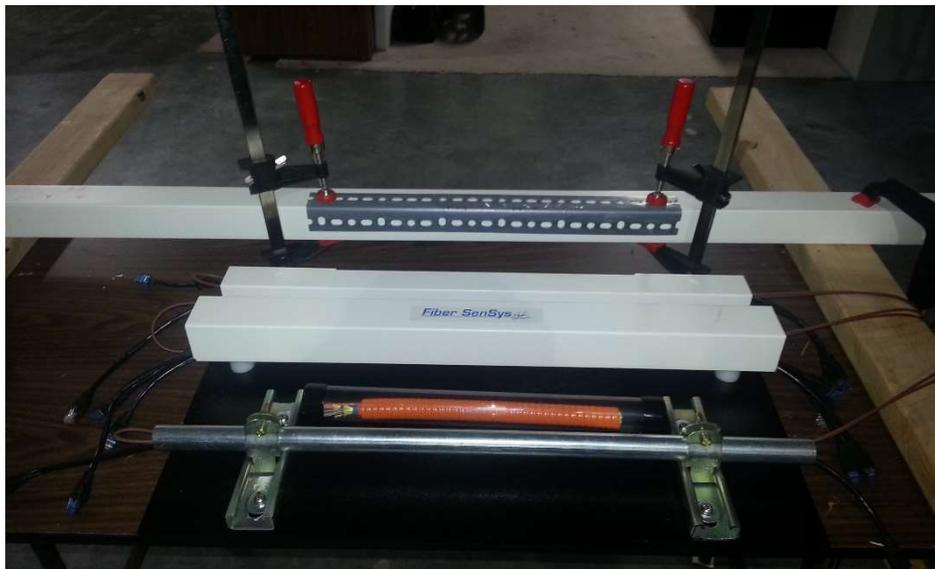
Sample testing setup using hardened raceway. The metal grating protects the raceway from being damaged during the testing process.
